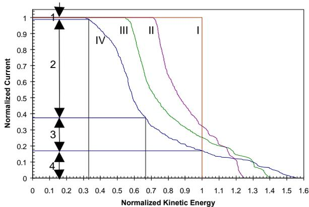
Fig. 1. Spent-beam analysis without rf drive (I) and at output power levels 475 W (II), 1258 W (III) and 2424 W (IV).
