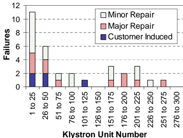
Figure 1 VKU-8891 series klystron failure data.
