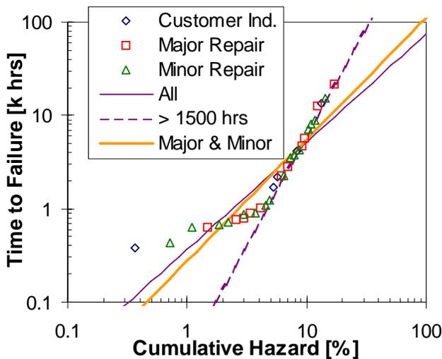
Figure 2 Weibull-hazard plot of VKU-8891 series klystron failure data.
